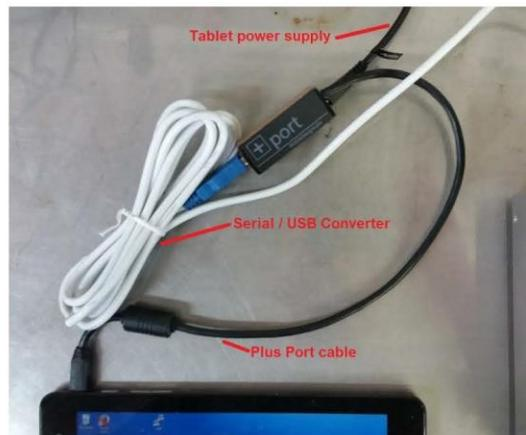
Figure 23: BMI Tablet/Plus Port Connection
